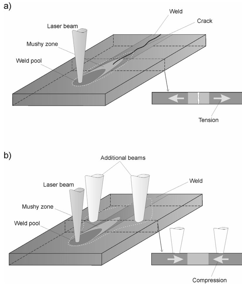
**Figure 1:** An initiation of the solidification crack in the mushy zone due to the transverse strain by the conventional laser welding (a) and prevention of the crack initiation due to the local heating by the multi-beam laser welding (b).
