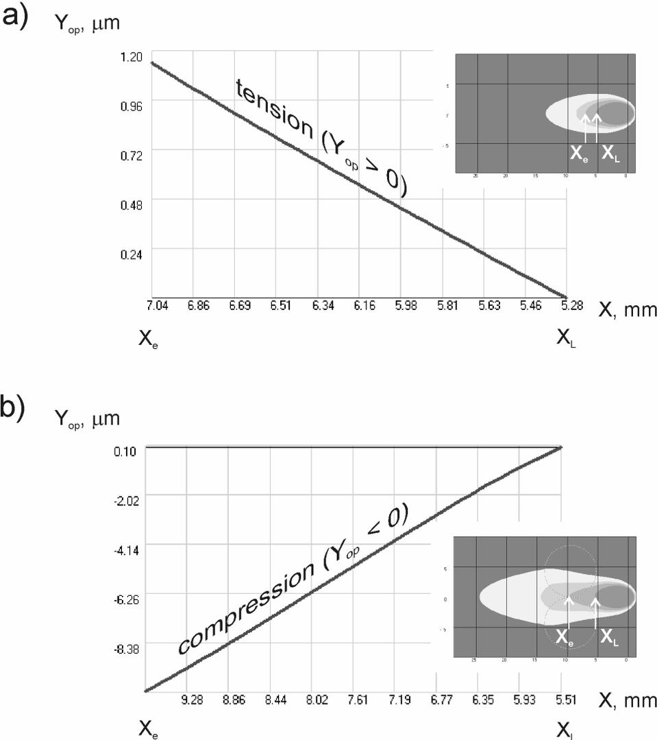
**Figure 5:** Calculated half values of the transverse strain accumulated in the mushy zone along the weld centerline for a weld produced (a) without and (b) with additional heating under the optimised parameters of the additional beams.
