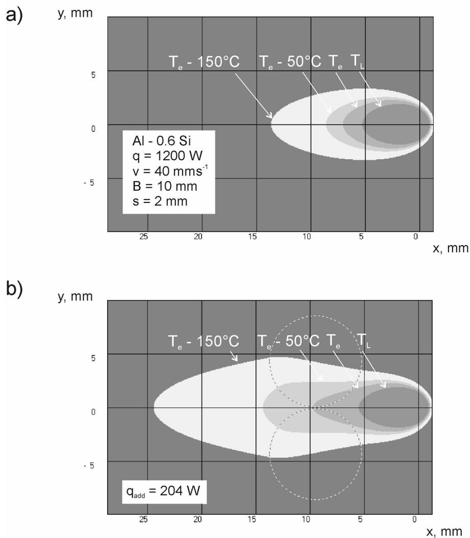
**Figure 4:** Calculated temperature fields for a weld produced (a) without and (b) with additional heating under the optimized parameters of the additional beams (the parameters of the main beam are constant for both cases).
