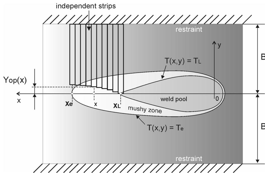
**Figure 3:** Schematical illustration of the strip expansion technique.
