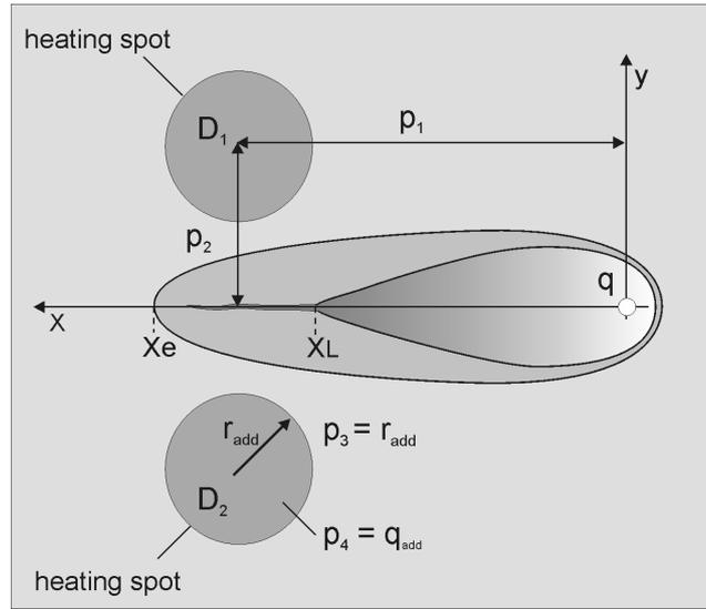
**Figure 2:** Parameters of the multi-beam laser welding.
